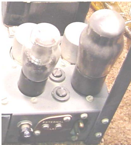
Above: beneath the power supply chassis – all neat and tidy (almost as new!). Below left: above view of the power supply chassis before cleaning – the 5Z4G on the right and VR150/30 on the left
