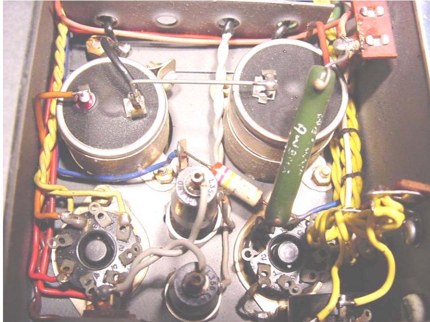
Above: beneath the power supply chassis – all neat and tidy (almost as new!). Below left: above view of the power supply chassis before cleaning – the 5Z4G on the right and VR150/30 on the left
